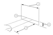
4. On the wall or screen you will observe a light pattern with high intensity flat segments at the top edge of the pattern. If the flat edges are not at the horizontal reference line, the beam will need to be adjusted.
